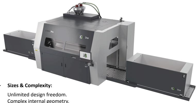
Using three-dimensional printing technology to create various sizes of complex molds and cores for a variety of industries. By selectively printing a specially-engineered binder into paper thin layer of foundry grade sand.
